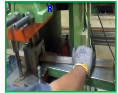
Die designed to cut in single stroke)
